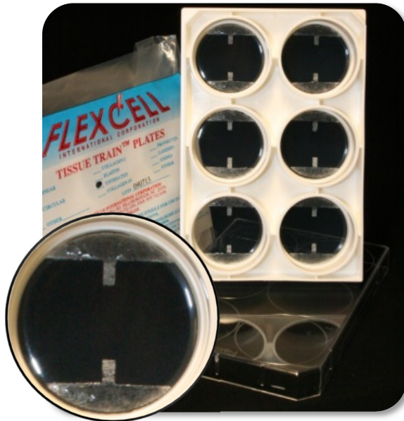
Figure 2. Linear Flexcell® Tissue Train® culture plate with non-woven nylon mesh anchors at north and south ends for gel-construct attachment.
